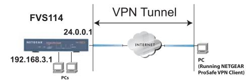
Figure 5-3: Client-to-gateway VPN tunnel
